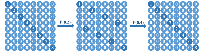
Fig. 2. One Example of Premultiplication and Postmultiplication by Stride Permutation on a Matrix
